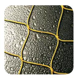
Lankoforce® netting is made from DSM Dyneema® fibre (Ultra High Molecular weight polyethylene). This netting is five times stronger than normal polyethylene and four than polyamide.
